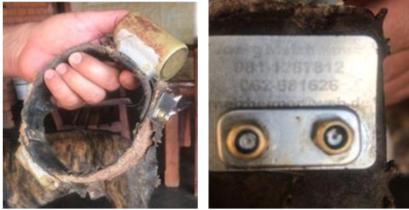
Figure 71: GPS radio collar belonging to IZW removed from an old male cheetah shot in a HWC incident.
